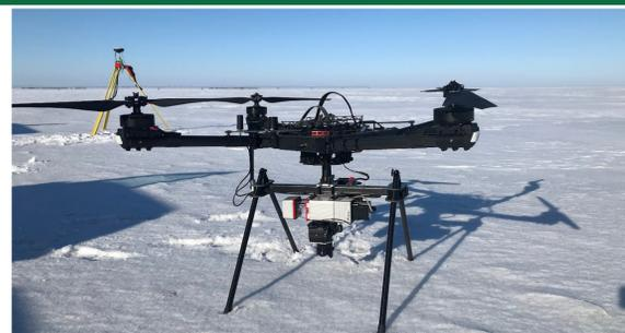
Figure 1: Riegl miniVUX-2UAV FreeFly AltaX UAV-lidar system
